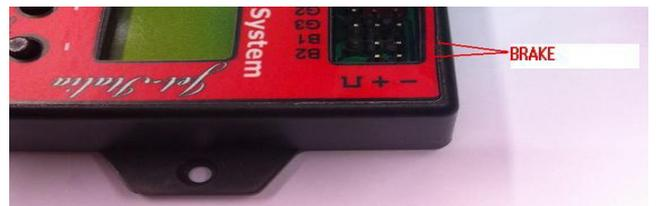
Please vertically plug in the left and right brake as shown above, no need to differentiate left or right.
