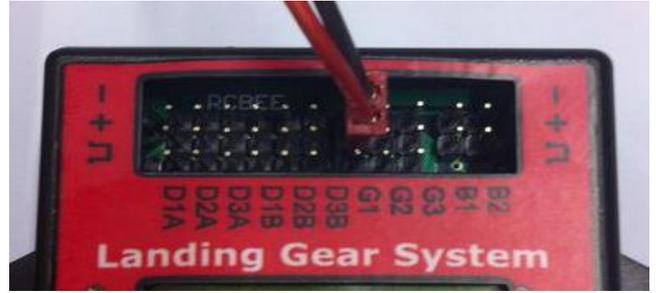
Please vertically plug the motor into the pins as shown above, and record the sequences. For example, 1 for front landing gear, 2 for left landing gear, 3 for right landing gear.
